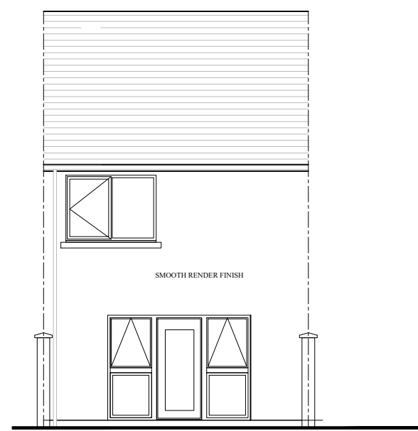
REAR ELEVATION (House Type B2 Terrace Unit)
